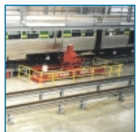
Railway Carriage Lift
