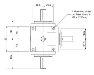
Tapped hole in end of each solid drive shaft - M6 x 16mm Deep
