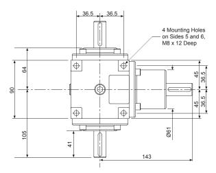
Tapped hole in end of each solid drive shaft - M6 x 16mm Deep
