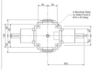
Tapped hole in end of each solid drive shaft - M8 x 25mm Deep
