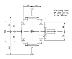
Tapped hole in end of each solid drive shaft - M8 x 25mm Deep
