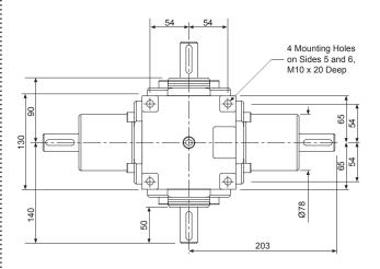
Tapped hole in end of each solid drive shaft - M8 x 25mm Deep
