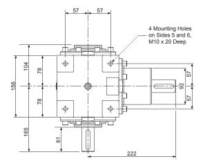
Tapped hole in end of each solid drive shaft - M10 x 25mm Deep
