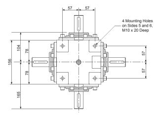
Tapped hole in end of each solid drive shaft - M10 x 25mm Deep
