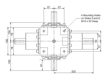
Tapped hole in end of each solid drive shaft - M10 x 25mm Deep
