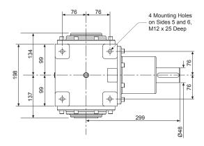
Tapped hole in end of each solid drive shaft - M12 x 30mm Deep
