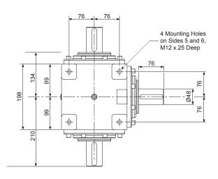
Tapped hole in end of each solid drive shaft - M12 x 30mm Deep
