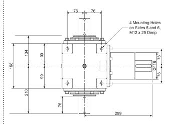
Tapped hole in end of each solid drive shaft - M12 x 30mm Deep
