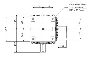
Tapped hole in end of each solid drive shaft - M16 x 38mm Deep
