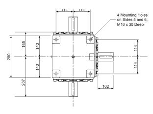
Tapped hole in end of each solid drive shaft - M16 x 38mm Deep
