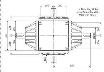
Tapped hole in end of each solid drive shaft - M16 x 38mm Deep
