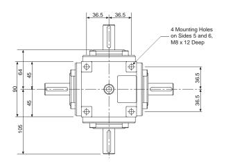
Tapped hole in end of each solid drive shaft - M6 x 16mm Deep
