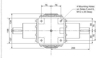
Tapped hole in end of each solid drive shaft - M12 x 30mm Deep
