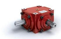
A gearbox is required for an Input Speed of 1000 rpm, an Output Speed of 500 rpm, an Output Torque of 150Nm and one Output Shaft. The Drive is by electric motor through a clutch mechanism and the gearbox is on the main drive of a heavy duty stacking machine. The machine operates for 10 hours per day, starts 8 times per hour and operates for 45 minutes in every hour, the other 15 minutes being taken up in loading the machine. The ambient temperature of the premises is 20°C.
