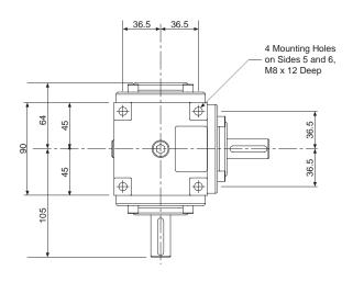
Tapped hole in end of each solid drive shaft -  $M6 \times 16 mm$  Deep
