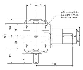
Tapped hole in end of each solid drive shaft - M10 x 25mm Deep
