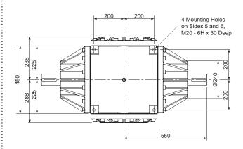
Tapped hole in end of each solid drive shaft - M16 x 38mm Deep
