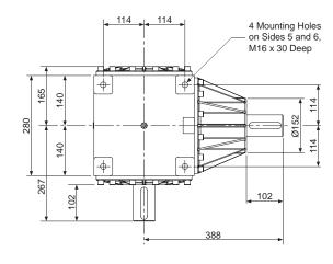
Tapped hole in end of each solid drive shaft - M16 x 38mm Deep
