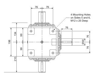
Tapped hole in end of each solid drive shaft - M12 x 30mm Deep
