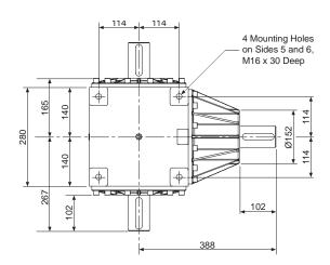
Tapped hole in end of each solid drive shaft - M16 x 38mm Deep
