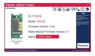
Quickly configure, test communication and calibrate Power Jacks wireless load cell devices.
